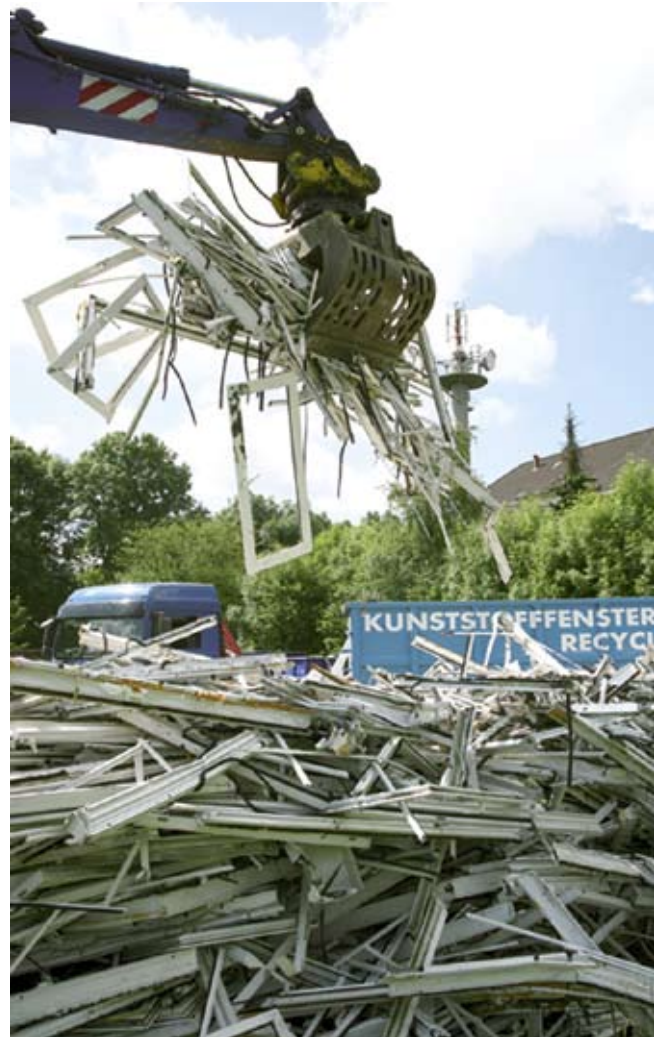
The collection and recycling of replaced PVC window systems is common practice today. At the end of the process, modern heat-insulating windows are manufactured which save energy and improve internal climate conditions.
